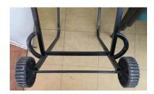
The trolley used to move stacks of chairs in the Main Hall at Calcot was difficult to use as the back legs of some chairs could fall down and rub against the trolley's wheels. A chair frame was used to make a stop to keep the chairs high enough over the wheels to prevent this happening.
